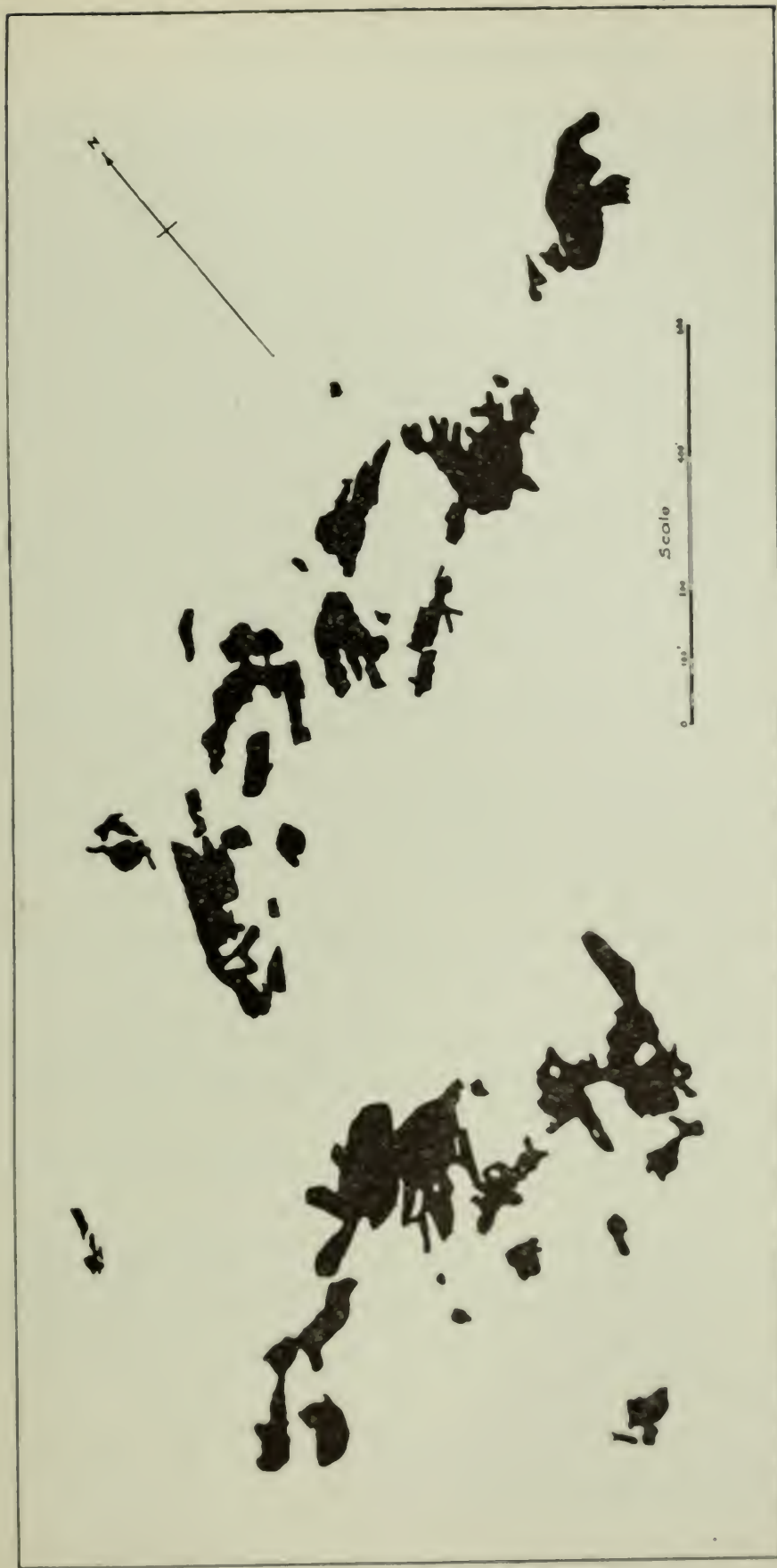
FIG. 28.—Plan of Ore-shoots in Jordan and "Highland" limestones, Old Jordan Mine, Bingham, Utah. (After Boutwell, U.S.G.S. Prof. paper 38, Plate XL.) These ore bodies show the preservation of the stratification of the enclosing rock in the ore. (On the original plate the stops are represented in out line and the mine workings are shown. The writer has constructed this plate by filling in the stops and omitting the workings.)
